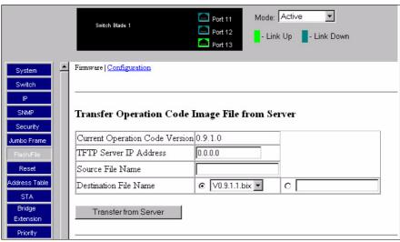
Figure 25: Transferring the new operation code image file
